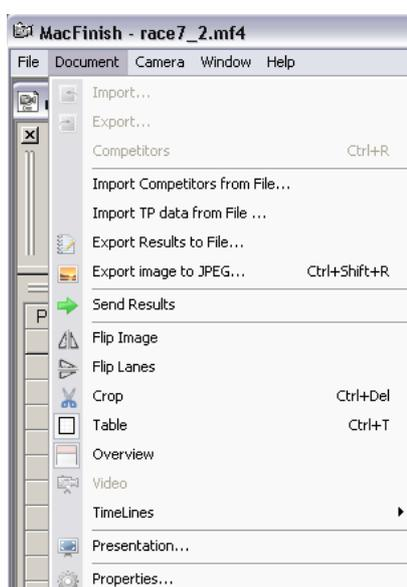
The top three menu selections of the "Document" menu are for the most interesting type; the two-directional data communication with a 'real' AthleticsManager. The following two items ('Send Results' and 'Export to File') are used for the 'simpler' one-directional transmission of data to a 'simpler' database program.
