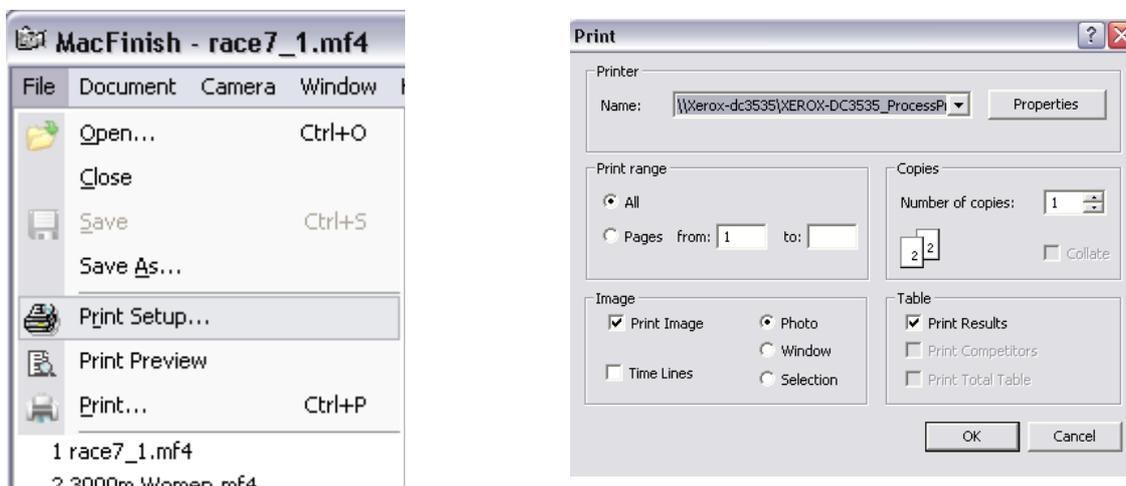
'Print setup' enables you to adjust your page (size, orientation, ...) for the printer.
