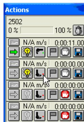
As soon as the start signal is given (starting pistol or manual push button), the timer starts running, the pistol-icon rotates to a horizontal position and its red led turns green. Also notice that the air shaft-icon is highlighted whenever a 'WindSpeed' apparatus is connected and if the wind speed measurement is selected (see parameter window). The wind speed can only be measured after the race has been started.
