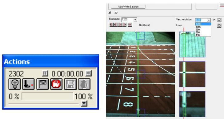
**WARNING for chapter 5.2 :** To use the 'scrolling' mode in the 'Scrolling camera view' window, the camera has to be 'active', this means that the 'Actions' window has to show a 'Ready' status (=before the race), **or** a 'Running' status (=during the race). In other words, the "lamp" icon should be visible in YELLOW color.
