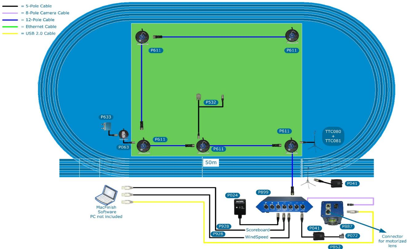
The schematic drawing above shows the mobile configuration with cable reels. With these 5 reels, you have ALL connections available at the 5 most important locations around the track. Similarly a fixed configuration can be made, if you replace the 5 cable reels with 12-wire underground cables and 5 removable connection boxes.
