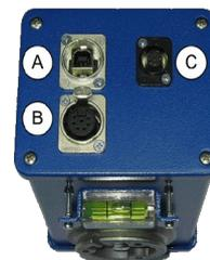
The next step is to connect the camera USB connector (top-left position "A" of the previous picture) with a USB connector of your PC, by means of the USB cable that we supplied with the system.
