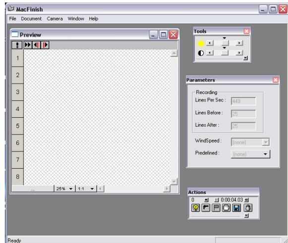
If you do not see the "Actions" window, try to (re-)connect the MacFinish camera by the menu-selection "Camera/Connect camera..". You should then get the "Connect" window, informing you about the "camera-ID" (=serial number of your camera(s)) that were found over the USB connection. Select the camera of your choice, and press the 'Connect' button.
