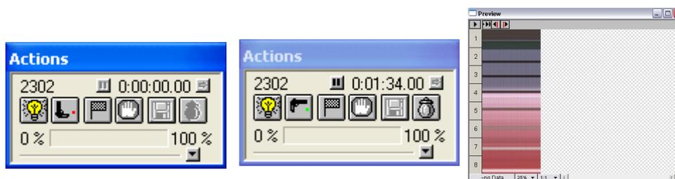
To record a "normal" image (not too dark or too light), we will need to give the MacFinish a "good" recording speed, for example 400 frames/second. If a lot of light is available; you can use more frames/sec, if it is very dark; use less. We will explain now how you can change the recording speed, and then further step by step how the camera direction can be corrected, and how the zoom, iris and focus of the lens can be adjusted.
