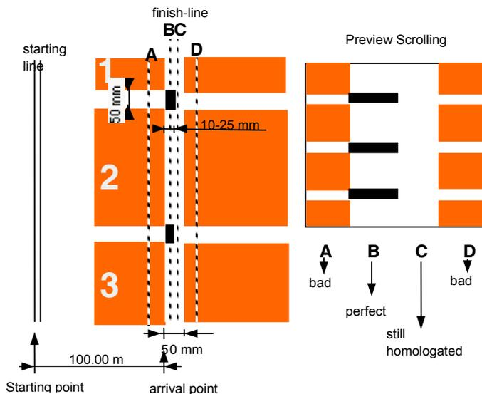
Now aim the camera at position B to get the best camera position! Use the '2D-view' mode in the camera window, or the 'Scrolling' mode in the Scrolling camera view window to find the correct camera position. A completely white background on a photo finish picture is also officially approved (for example for World Record) as the athlete then has run a few cm too much, but it is far less recommended in the interest of the athlete!
