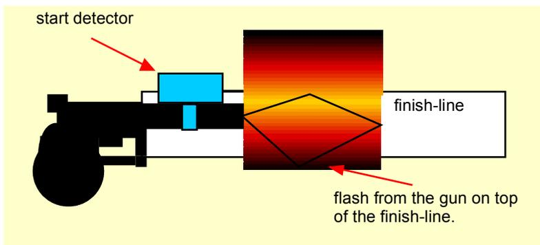
As soon as the sensor(s) inside the start detector register the explosion, time will start running within 0.5 microseconds after the starting shot. This should coincide with the camera registration of the flash from the starting pistol:
