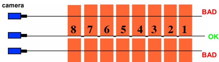
3. Adjust vertical angle of the camera + zoom of the lens.
