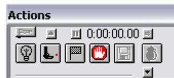
If a start signal is given, the air sock icon becomes highlighted and the MacFinish operator can now click it in order to start a 10 seconds wind measurement. The shortcut to do this is the "F12" key on the keyboard (if enabled).
