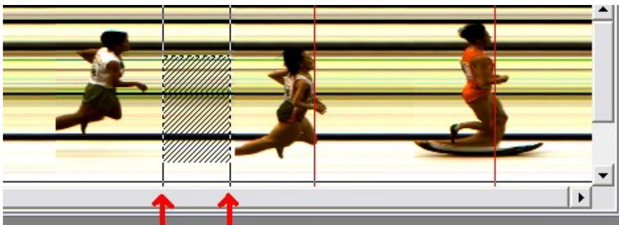
We have selected a part that we wish to cut (between the two vertical lines) by pointing with the mouse, press the mouse button, move the mouse and release the mouse button. Now we select 'Crop' under the 'Document' menu. It will remove the part that we wanted to cut out, but this will have no influence however on the time display for the participants.
