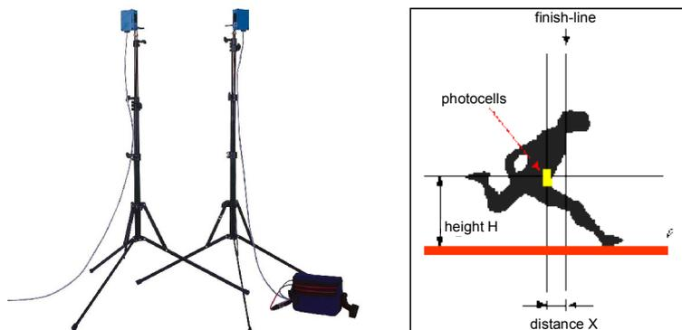
Try to position the photocells as close as possible to the finish line, but make sure that they do not obscure the view of your camera(s) !
