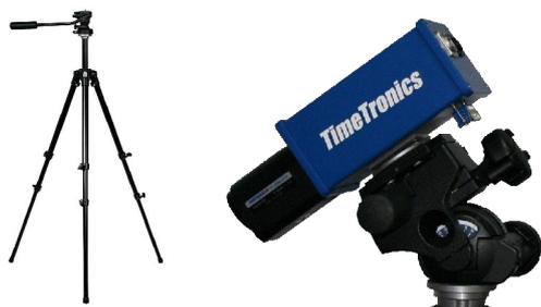
Now attach the camera head on the tripod or camera pole.
