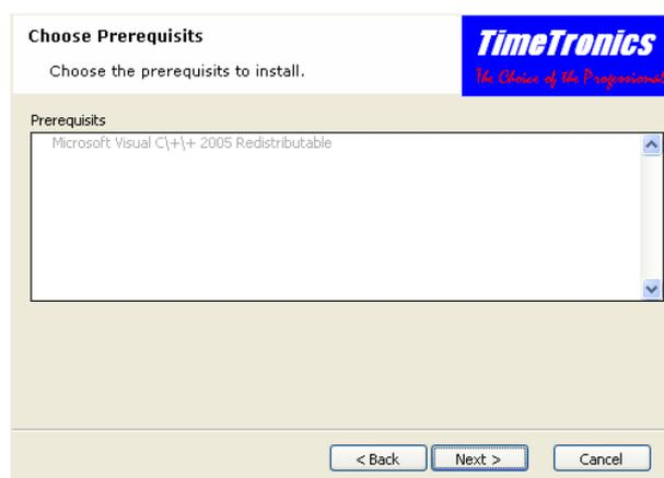
First the prerequisites will be installed. A prerequisite is a software component that has to be installed before MacFinish can run. For MacFinish2D version 8.0.x the only prerequisite is Microsoft Visual C++ 2005 Redistributable. If it is already present on your computer, it will be grayed (like in the image above).
