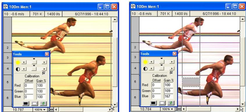
Now you can also calibrate the 'black offset'. Select a 'black' part on the photo and click the black rectangle on the bottom of the 'Tools' window. After you have done this, the new values under 'Gain' and 'Offset' will be automatically displayed.
