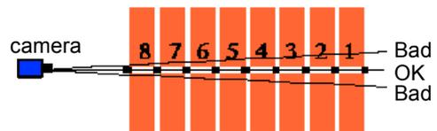
The camera is positioned correctly (**for athletics T&F**) when the image in the 'Scrolling camera view' window is white with black horizontal lines.
