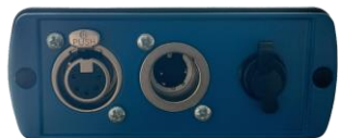
Wireless Start - Starter unit (Bottom) - 5P connection for Start - 5P connection for Service - Connection for Charger
